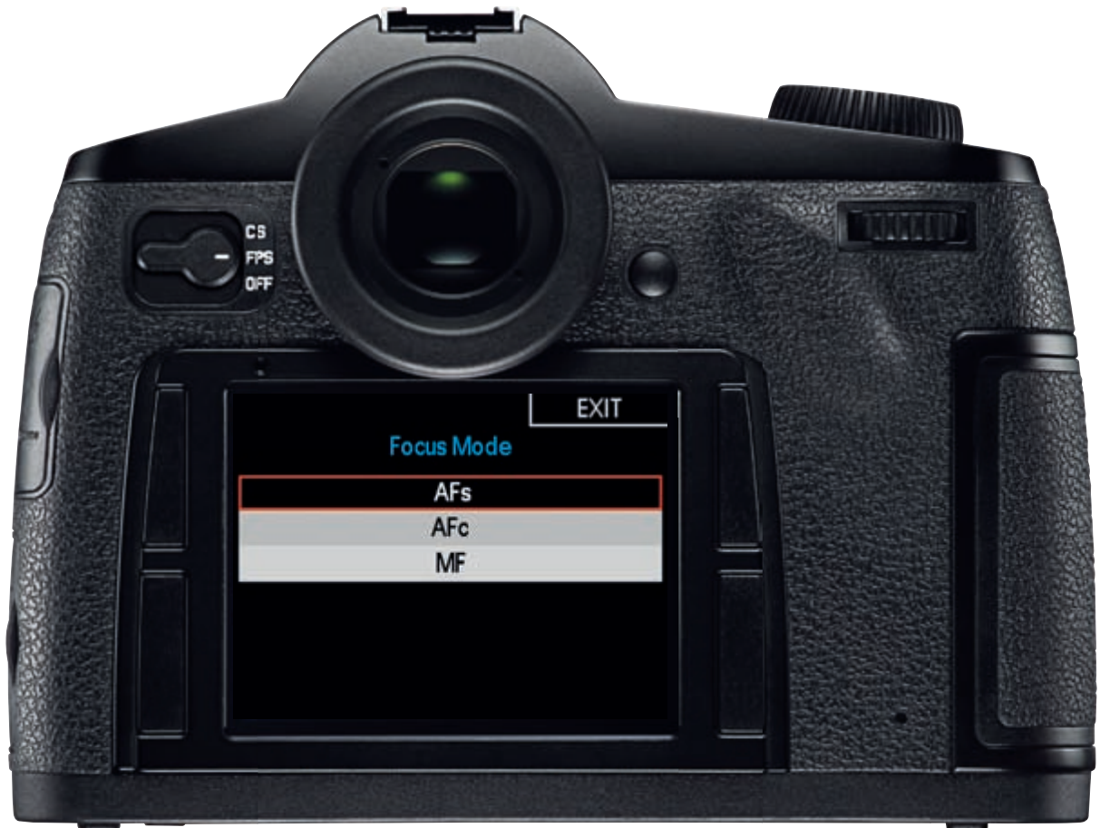
Flexible changeover from autofocus with focus or release + focus priority and manual focusing (full-size view).
