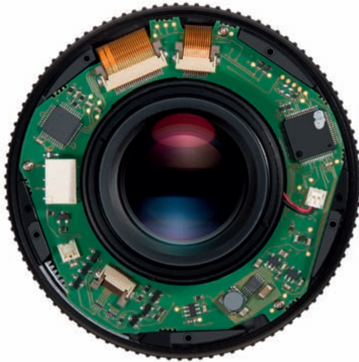
In the S-System, focusing is controlled by the built-in 'brain' of each lens.
