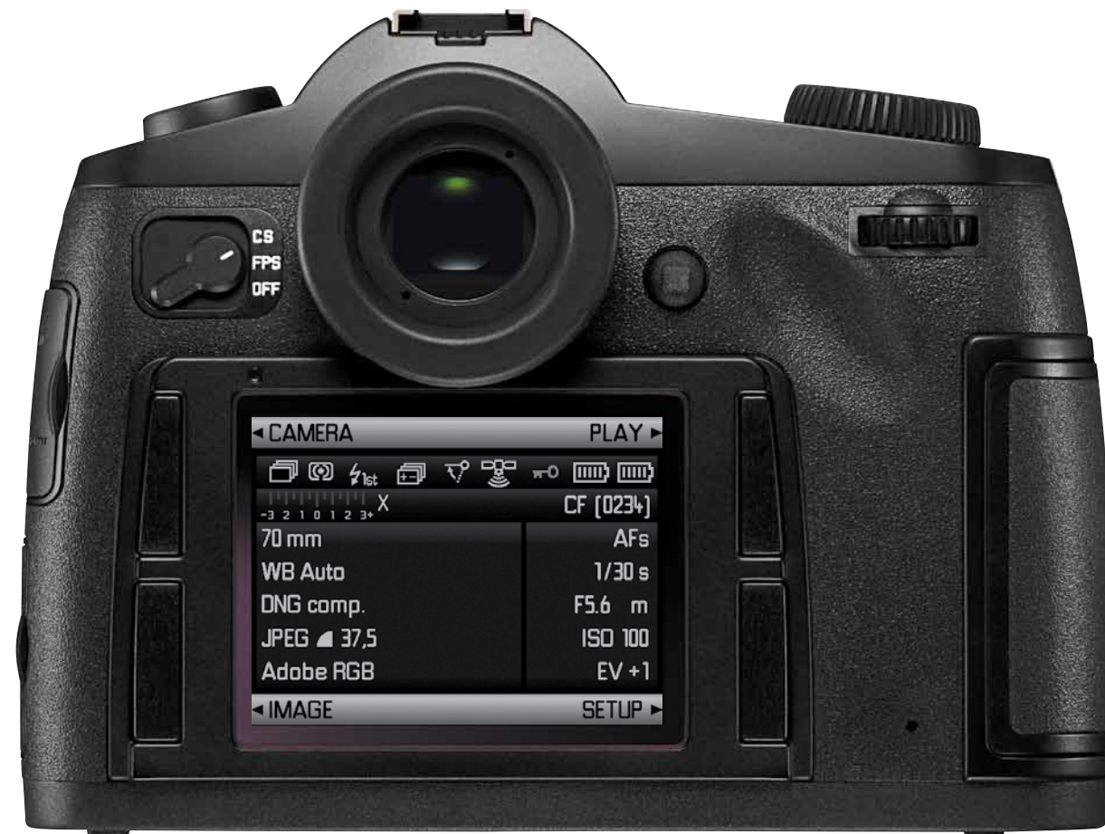
In combination with only four programmable buttons and a mini-joystick, the clearly structured menu guarantees fast and intuitive control of all camera functions. (Full-size view)
