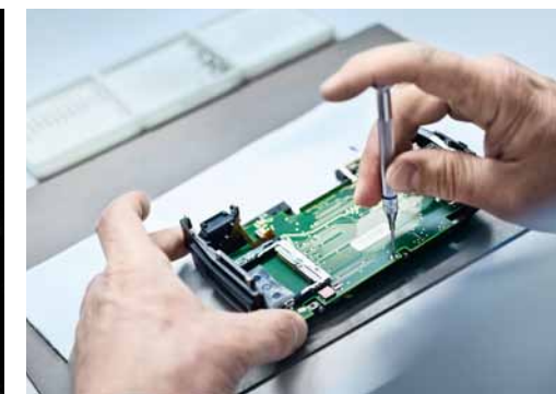
Installation of the control board on the rear shell of the Leica S2.
