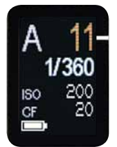
A glance at the OLED panel on the top deck of the Leica S shows its user the most important camera settings with commendable clarity. (Full-size view)
